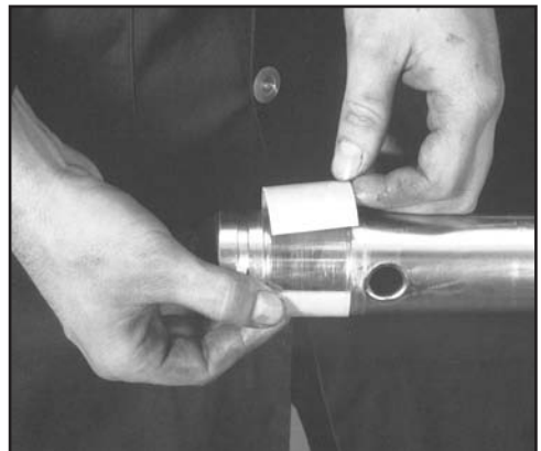
FIG. 73: POSITION REAR SLIDE TAPE
