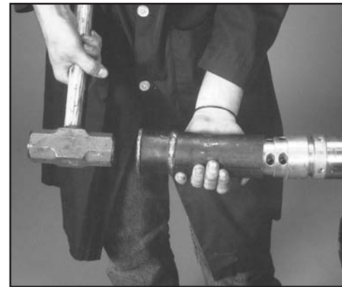
FIG. 31: USING PIPE TO SECURE STEPPED CONE
