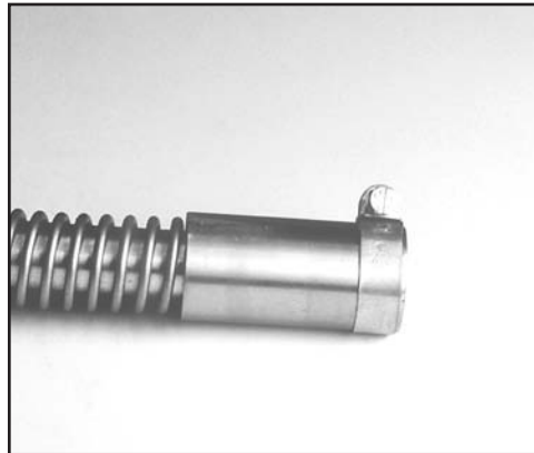
FIG. 47: REFORM WITH COMPRESSION CLAMP
