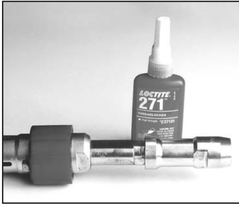
FIG. 51: APPLY LOCTITE AND TIGHTEN CONTROL STUD ADAPTER
