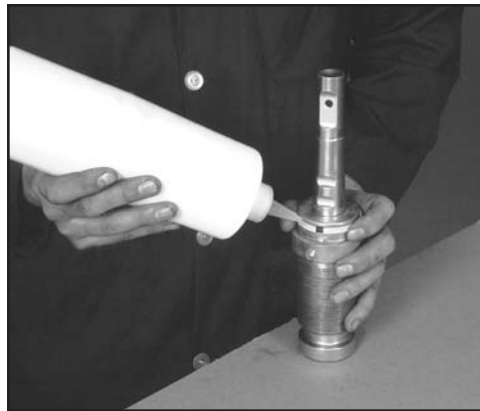
FIG. 30: GREASE THE SEAL
