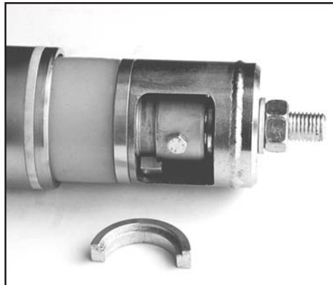
FIG. 62: REMOVE SEGMENTED RINGS
