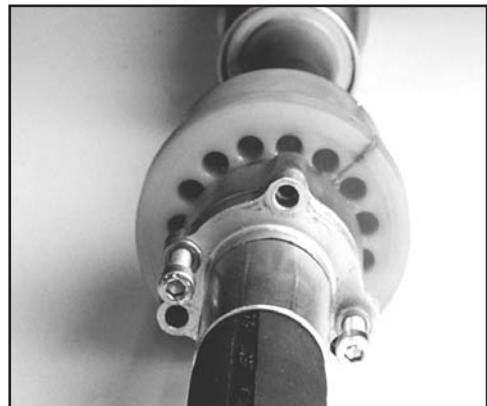
FIG. 58: 2 SCREWS USED AS JACK SCREWS
